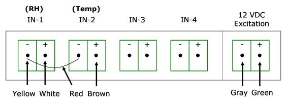
The probe must be defined in the fourtec software using the following output values:
